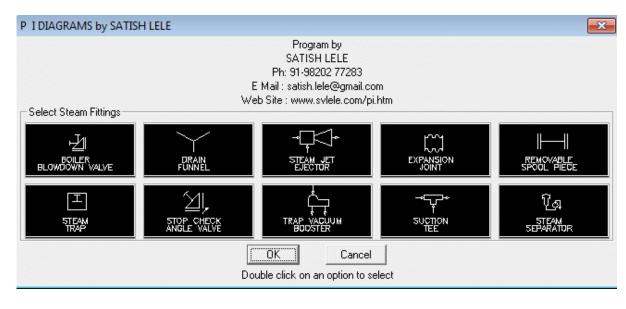
**Dialog Box to insert Pipe Fittings**: We can insert Pipe Fittings in the drawing. We select a Pipe Fitting to be inserted. We are then asked to select a line at left insertion point where Pipe Fitting is to be inserted. Pipe Fitting is put on the layer of the line.
